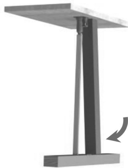
C&D: Fasten locator block to floor with appropriate screw type.
